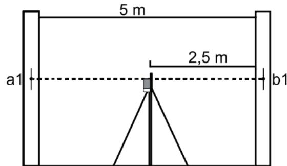
Set up the instrument 0,5-0,7m away from the wall and make, as described above, the same marks. If the difference  $\{a_1-a_2\}$  and  $\{b_1-b_2\}$  is less than the value of "accuracy" (see specifications), there is no need in calibration.
